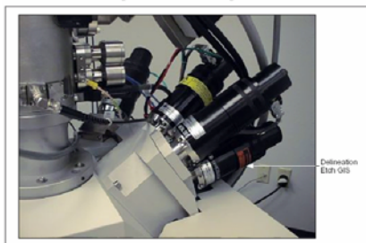
Figure 6 200 Series Port Configuration
